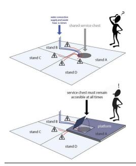
Whenever a service chest is shared between more than one stand in one island, it must remain accessible at all times (through a hatch).
