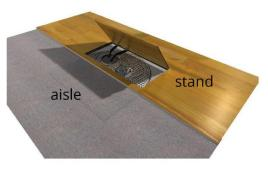
Whenever a service chest is half covered by a division wall or is at the limit of the stand, the area around the chest must remain accessible.
